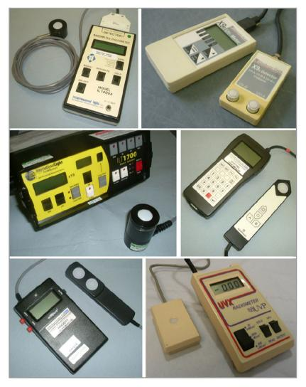
Fig 3. Examples of ultraviolet radiometers.
