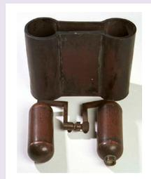
*Gas cylinders and calorimeter used by Joule to demonstrate that expanding gases have a cooling effect - the principle used in refrigeration.*
